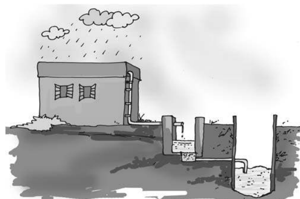
Fig. 14.13 Rooftop rainwater harvesting
