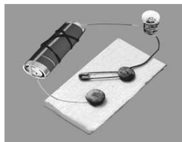
Fig 12.9 An electric circuit with a switch
