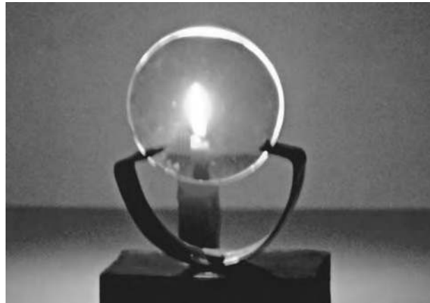
Fig. 15.27 Image formed by a concave lens
