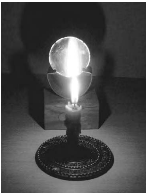
Fig. 15.16 Virtual image formed by a concave mirror
